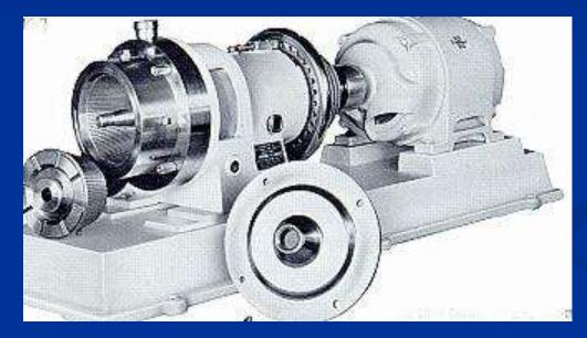
G100 25 tph with 100 HP motor G125 40tph with 125 HP motor
